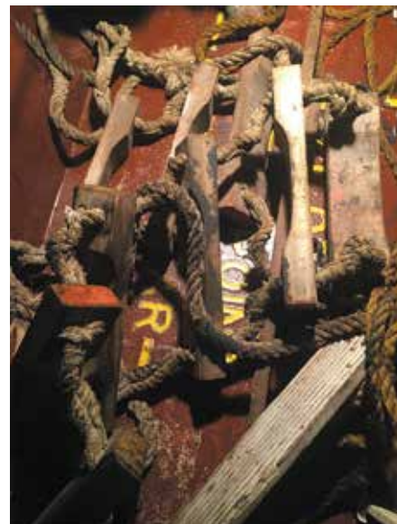
Figure 1 Starboard pilot ladder covered in HFO
