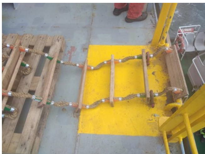
Fig 2: Using D-Schackles will damage the pilot ladder
