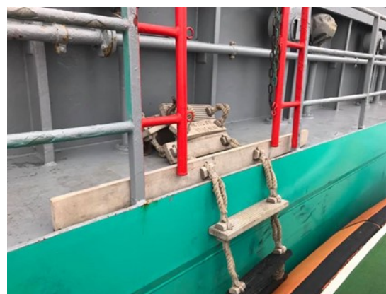
Fig 4: Using the spreader as a securing device
