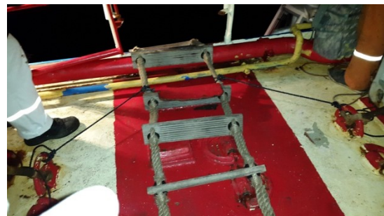
Fig 3: The shoestrapping method of securing
