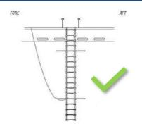
Finally, when a retrieval line is rigged, it shall be rigged at or above the bottom spreader and lead forward to prevent possible snagging at the pilot launch.
